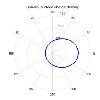
We can also show the induced charge distribution in a polar plot. The direction of the X axis is given when the angle is 0°.
