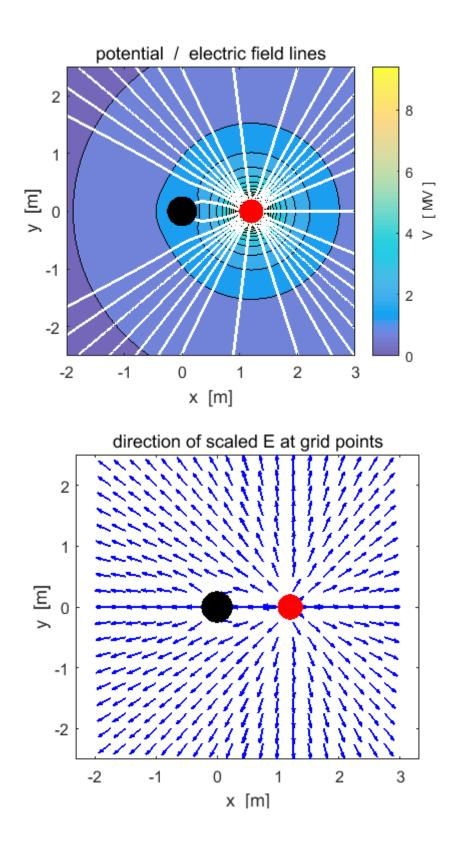
The uncharged sphere is insulated, therefore its charge must remain zero in the electric field due to the point charge and the surface of the conducting sphere is an equipotential surface. In an electric field free region, the potential at the surface of the uncharged sphere is zero. In the presence of the electric field created by the point charge, the potential at the surface of the sphere is raised to 1.5 MV.
