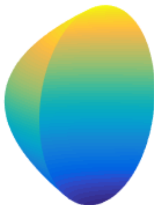
Fig. 4. A [3D] plot showing the outer surface of the solid of revolution. The Matlab functions cylinder and surf were used to generate the [3D] plot.
